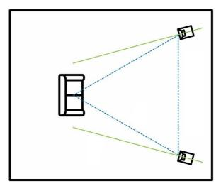
If a symmetrical position is impossible and the distance from each speaker to the listening position is different, then this can be compensated digitally by adjusting the setup in the processor. The speaker should be moved back following the guide-lines for toe-in.
