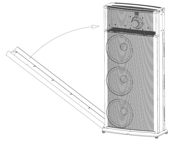
Secure the panels by the Allen bolts fixed in the frame (Hex4)
